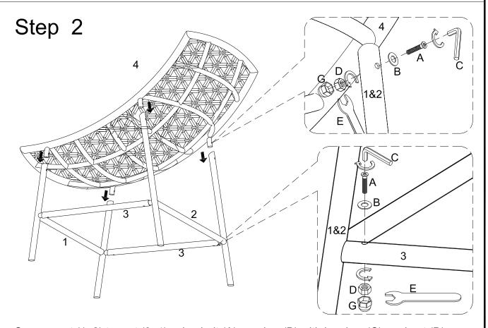
Secure part (1, 2) to part (3, 4) using bolt (A), washer (B) with hex key (C), and nut (D), screw cap (G) with wrench (E).
