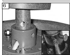
Install downrod with canopy and yoke covers into yoke. Align hole in downrod and yoke, push pin through and replace keeper. Tighten set screws and locking nuts (see inset).
