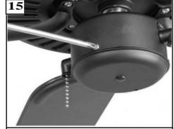
Remove the 3 screws in round holes. Remove cap by twisting and pulling down. Save screws.
