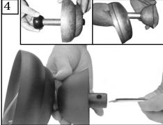
Install downrod to canopy and then install yoke cover to downrod. Thread wires and safety cable through downrod
