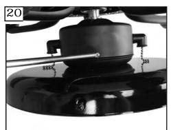
Attach switch cap to fan by lining up 3 screw holes and twisting cap clockwise. Then tighen the 3 screws.
