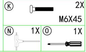
Warm Tip: Please don't tighten screws before finish assemble.
