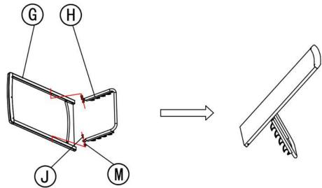
Please note: The Plastic cylinder Part M must be between Part G and Part H.
