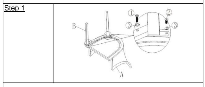
Open the carton and place all the parts onto a clean, non-marring surface. Attach the Right Leg(B) to Seat(A) using Bolts((1)) and Washers((3)) with Allen Key((4)) as shown above.
