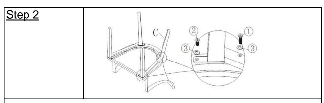
Attach the Left Leg(C) to Seat(A) using Bolts(①) and Washers(③) with Allen Key(④) as shown above.
