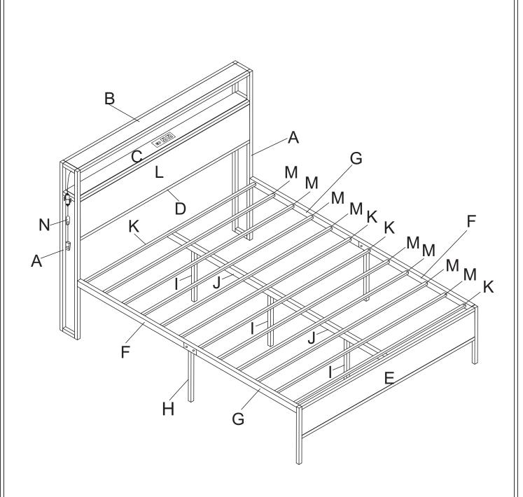
Notice: Do not tighten the screws too tightly at the beginning of the assembly. After each hole position is matched well, with gently force to screw, if there is no problem, then tighten all the screws.
