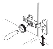
Screw C for door up & down adjustment.
