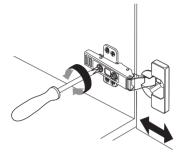
Screw A for door in & out adjustment.
