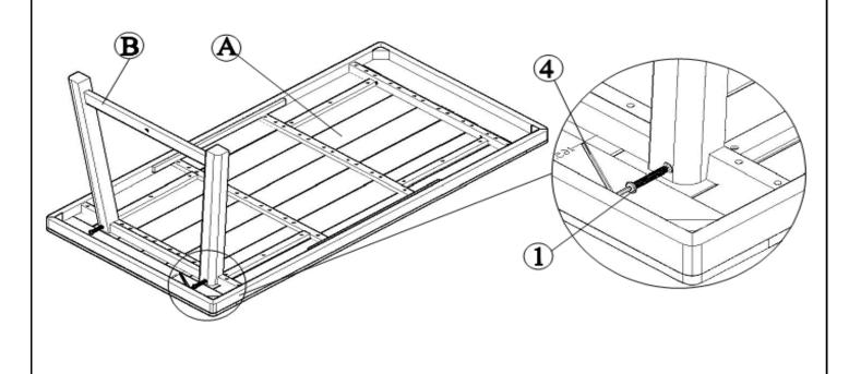
Attach Leg Panel(B) to Table Top(A) using Bolts( $\widehat{1}$ ) with Allen Key( $\widehat{4}$ ) as shown above.
