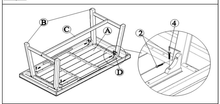
Align the Corner Blocks(D) to the Table Top(A) and Leg Panels(B) and attach using Screws( $^{\circ}$ 2) with Allen Key( $^{\circ}$ 4) as shown above.
