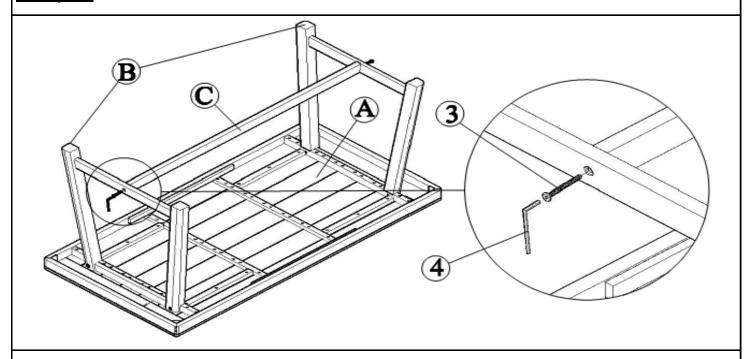
Insert the tenons on the Leg Support Bar(C) into the mortises of the Leg Panels(B). Attach Leg Support Bar(C) to Leg Panels(B) using Screws( $\mathfrak{F}$ ) with Allen Key( $\mathfrak{F}$ ) as shown above.
