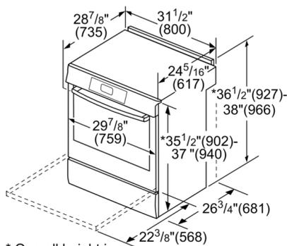
\* Overall height is adjustable via leveling legs.
