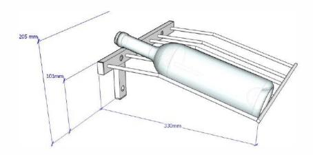
The presentation style rack is available in 9 wide (990mm) or 3 wide (330mm) versions We recommend a minimum vertical spacing of 205mm per row when installing multiple racks Multiple units can be joined to create single display
