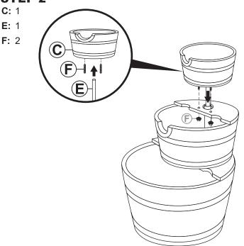
Install two Grub Screws (F) into Top Barrel (C). Then, firmly attach Water Tube (E).
