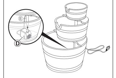
Place Electric Submersible Pump (D) in the bottom barrel. Run the power cord through the hole in the back of the barrel. Firmly connect the pump to the water tube.
