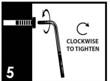
Make sure all parts are properly aligned, then use the appropriate hand tool to completely tighten the bolts or screws. Do not use power tools and do not overtighten.
