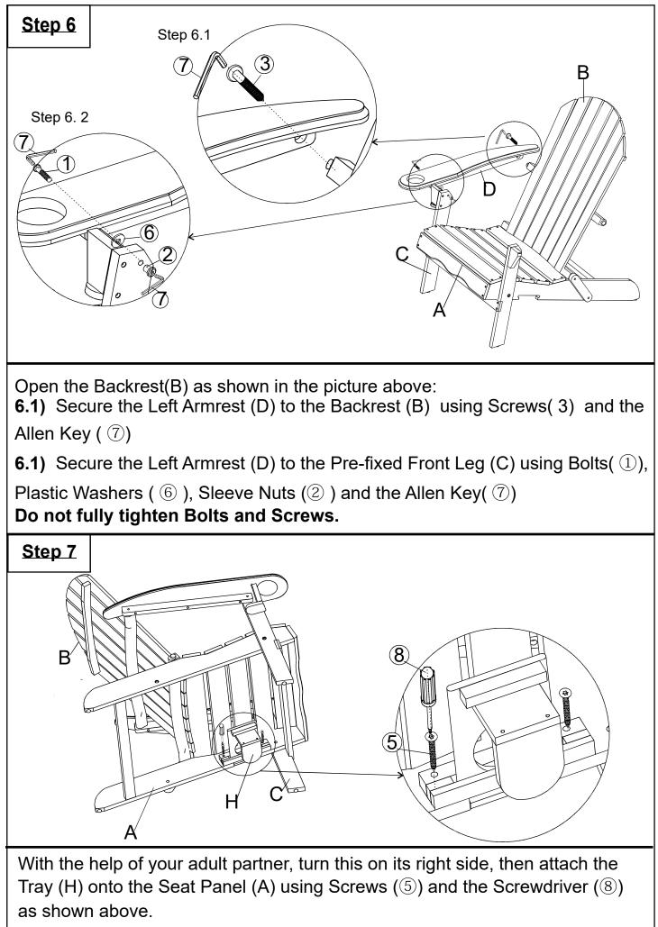
Do not fully tighten Screws.
