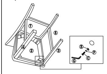
Using the allen key(G) to fasten 4pcs bolt(C) and 4pcs flat washer(E) and 4pcs spring washer(F).
