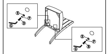
Open the velcro strips on the edge of the seat frame, attach the seat frame (2) to the backrest (1), using the allen key (G) to fully fasten 6pcs bolt (B and D), 6pcs flat washer (E) and 6pcs spring washer (F).
