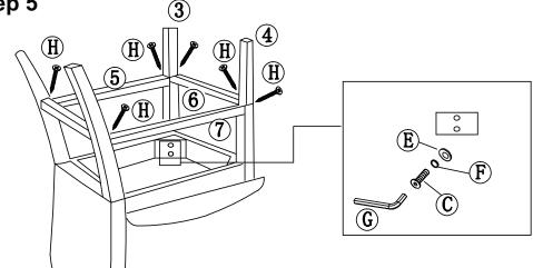
Secure with 6pcs selftapping screw(H) as showed in above figure. Note: If you have trouble inserting the strechers, loosen the bolts slightly to allow for extra space. Turn stool upright on its legs and place on a flat, level floor, make sure that the stool is level and square. Tighten all the bolts completely with Allen key(G).
