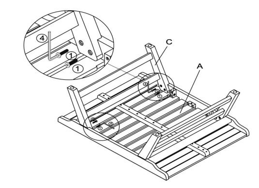
Attach the remanning Leg Frame(C) to Seat Panel(A) using Bolts(1) with Allen Key(4). **Do not fully tighten the Bolts.**
