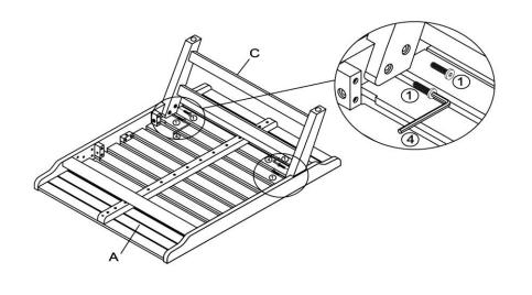
Place Seat Panel(A) facedown on a clean, non-marring surface. Attach Leg Frame(C) to Seat Panel(A) using Bolts(1) with Allen Key(4). **Do not fully tighten the Bolts.**
