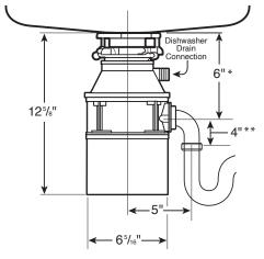
$^{\ast}$  Distance from bottom of sink to center line of disposer outlet. Add 1/2" when stainless steel sinks are used.
