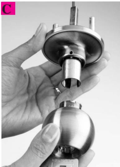
Apply pressure to the rose with your thumb and forefinger, and pull the knob off the spindle.
