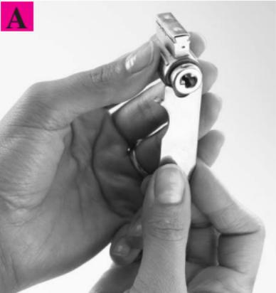
Re-insert the key into the plug. Use the end of the removal tool to push the clip out.
