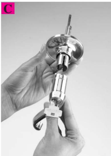
Apply pressure to the rose with your thumb and forefinger, and pull the lever off the spindle.
