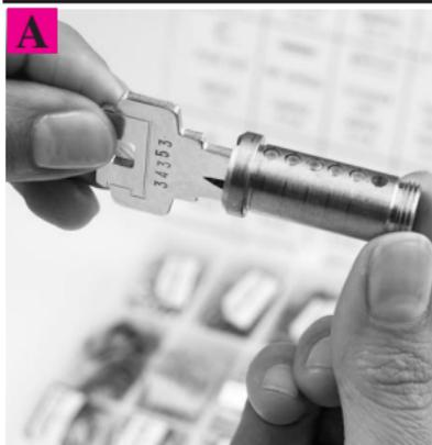
Use the numbers on the key bow or the key gauge to determine a new combination. Insert a new key completely into the key plug.
