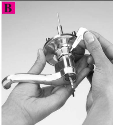
Use the lever catch tool to depress and release the lever catch.
