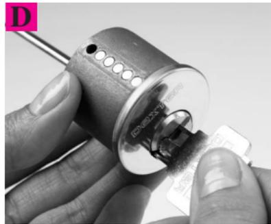
Reinsert and turn key to ensure cylinder is working properly. In the event of binding, loosen or tighten the cylinder cap until the cylinder works smoothly.
