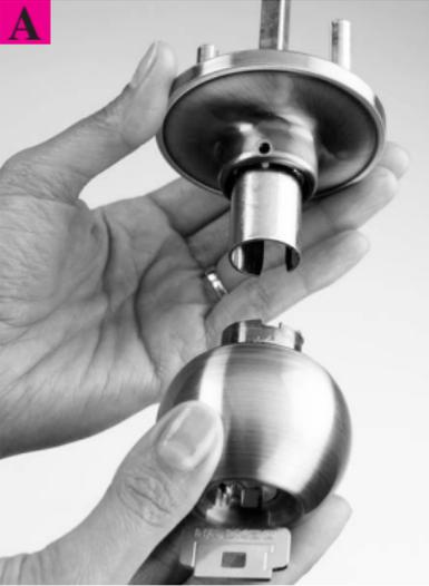
Align the slot of the knob shank and rollback. Push the knob all the way back until the knob is firmly retained by the knob catch.
