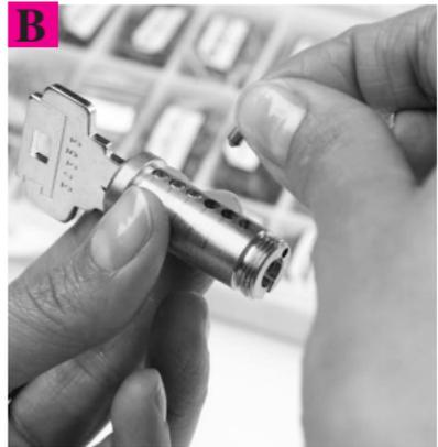
Load the new pins into the cylinder plug with pins from the rekeying kit that correspond to the new key combination.
