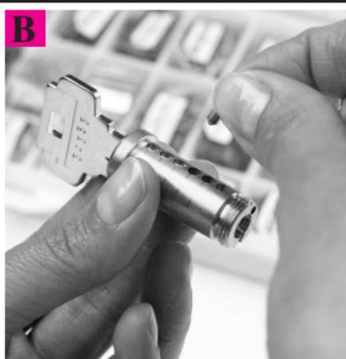
Load the new pins into the cylinder plug with pins from the rekeying kit that correspond to the new key combination.
