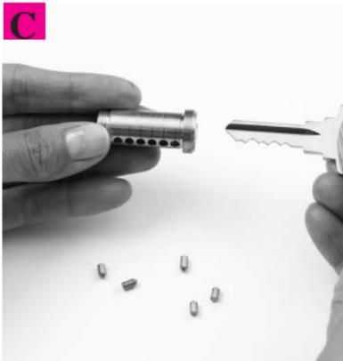
Empty the bottom pins from the cylinder plug and remove the old key.
