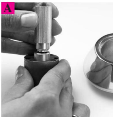
Match the grooves on the cylinder cap with the teeth on the cylinder cap removal tool.
