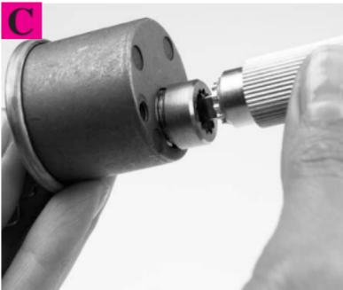
Screw on cylinder cap and driver with the cylinder cap removal tool.
