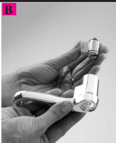
Remove the key from the cylinder and remove the cylinder from the back of the lever.
