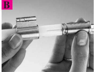
Hold the follower bar firmly against the cylinder plug and carefully slide it through the cylinder body until the plug and the front of the follower have passed completely through the cylinder body.
