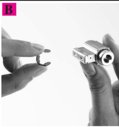
Remove the clip with the hook of the removal tool.
