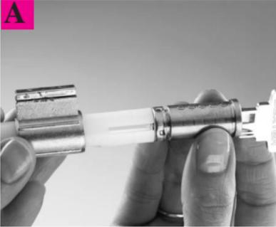
Turn the key to the 3:00 position. Push on the follower bar to reinsert the cylinder plug into the cylinder body.
