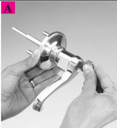
Insert the key into the cylinder (with teeth of key facing up). Turn the outside lever counter-clockwise until the lever catch is visible and aligns under the lever catch hole (as shown).
