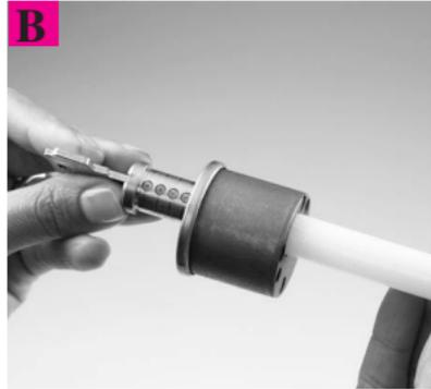
Hold the follower bar firmly against the cylinder plug and carefully slide it through the cylinder body until the plug and the front of the follower have passed completely through the cylinder body.
