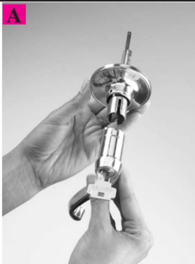
Align the slot of the lever shank and rollback. Push the lever all the way back until the lever is firmly retained by the lever catch.
