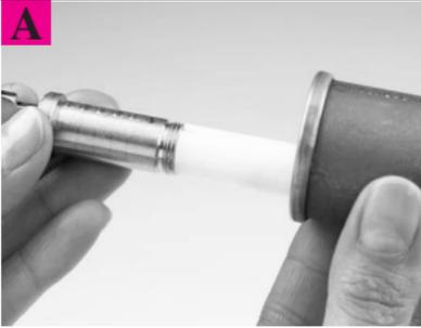
Turn the key to the 3:00 position. Push on the follower bar to reinsert the cylinder plug into the cylinder body.
