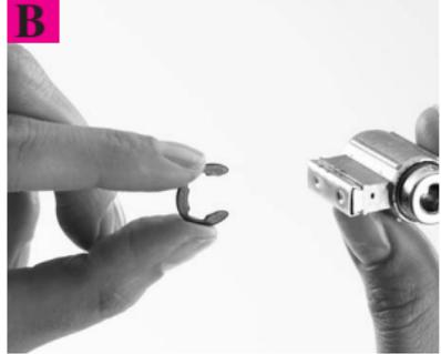
Reattach the retaining clip to the back of the cylinder plug by pushing it into the groove until it snaps back into place.
