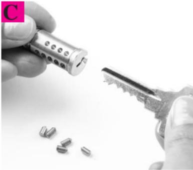
Empty the bottom pins from the cylinder plug, and remove the old key.
