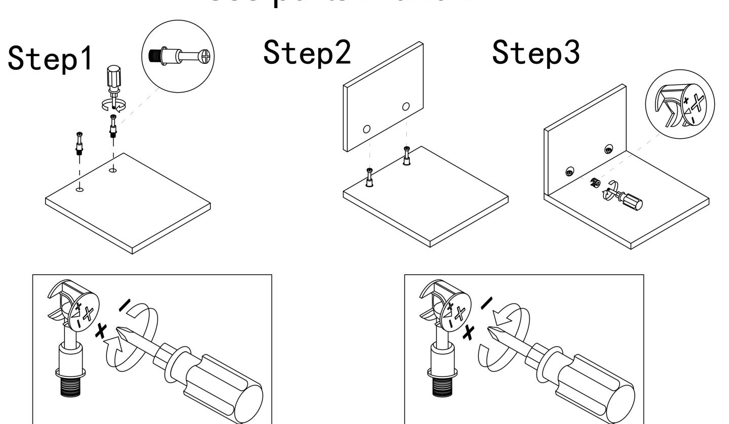
Use a screwdriver to lock in the direction of the "+" sign Disassemble along the direction of "-" sign
