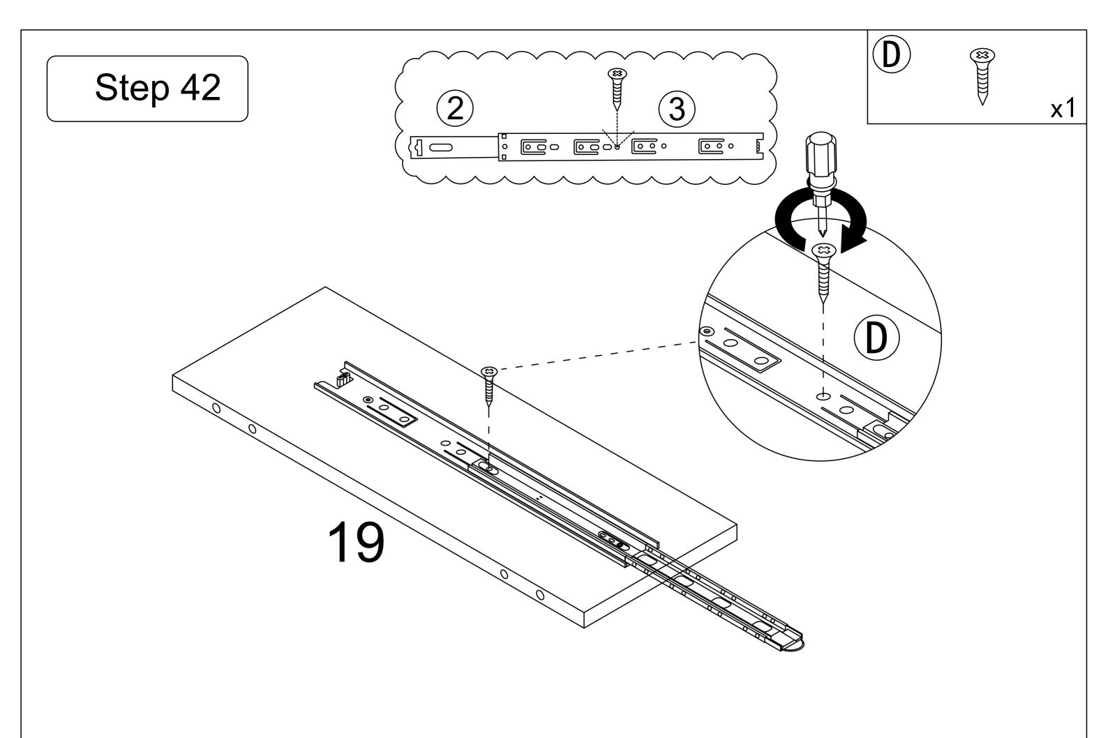
On the left side of the No. 19 plate, pay attention to the direction when installing
