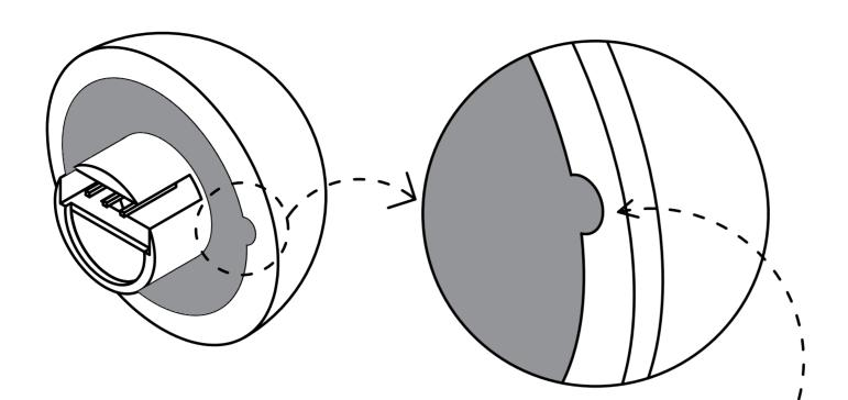
Remove the film before installation
