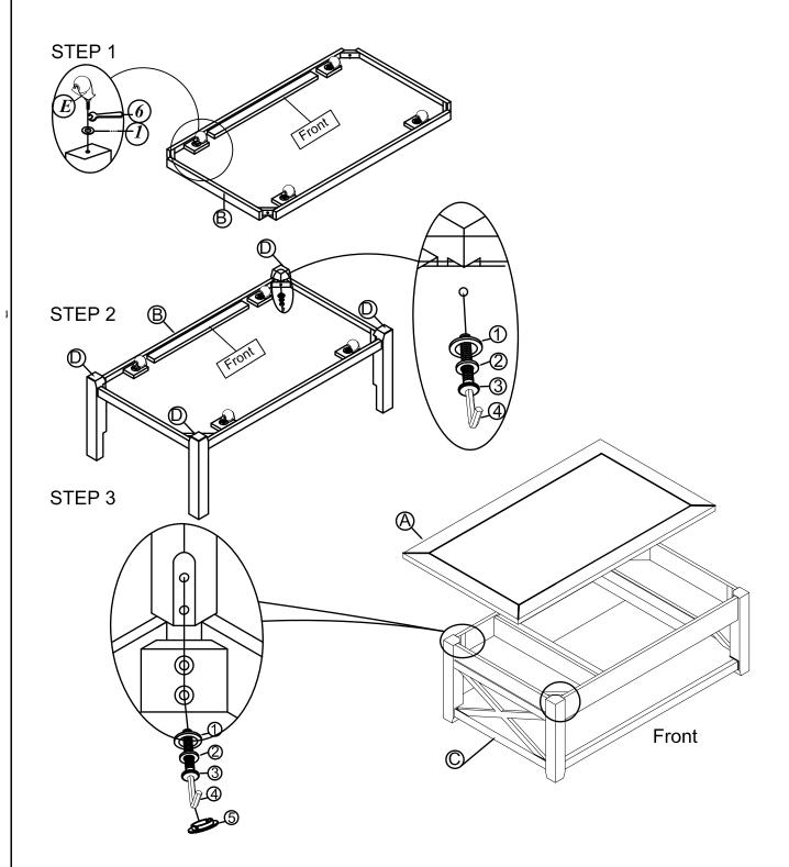
Step 1: Place the Bottom Shelf (B) upside down on the floor with a piece of cloth or carpet underneath to prevent finish from scratching. Attach the Caster (E), to the holes of Bottom Shelf (B), by inserting Flat Washer (1), and secure with Wrench (6).
