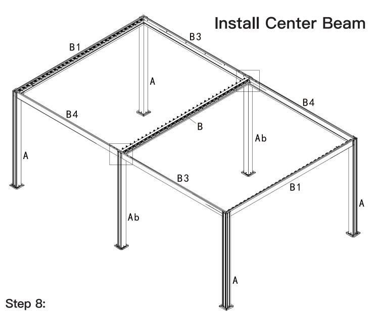
Place Part #B on the middle joint of Part #B3 and Part #B4 with 4 Bolts 1# as shown. Repeat the above procedures to assemble another side.
