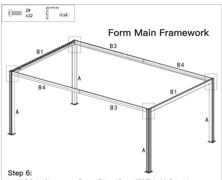
Install 8 Bolts 2# to secure Beam #B1 and Beam #B3/B4 with Post #A, then install Part #G into Corner Post #A as shown.
