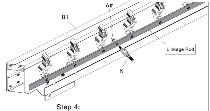
Insert Part #K into the hole on Linkage Rod of Beam #B1. Secure with Nut 6# and gasket as shown.
