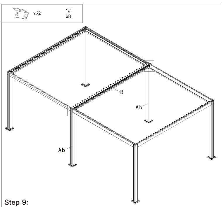
Connect Part #B and Part #Ab with Part #Y and secure with 4 Bolts 1# as shown. Repeat the above procedures to assemble another side.
