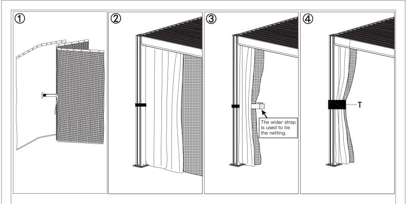
The small netted straps on the netting are needed to cross the hole on the curtains, then tie the small netted strap on each post.
