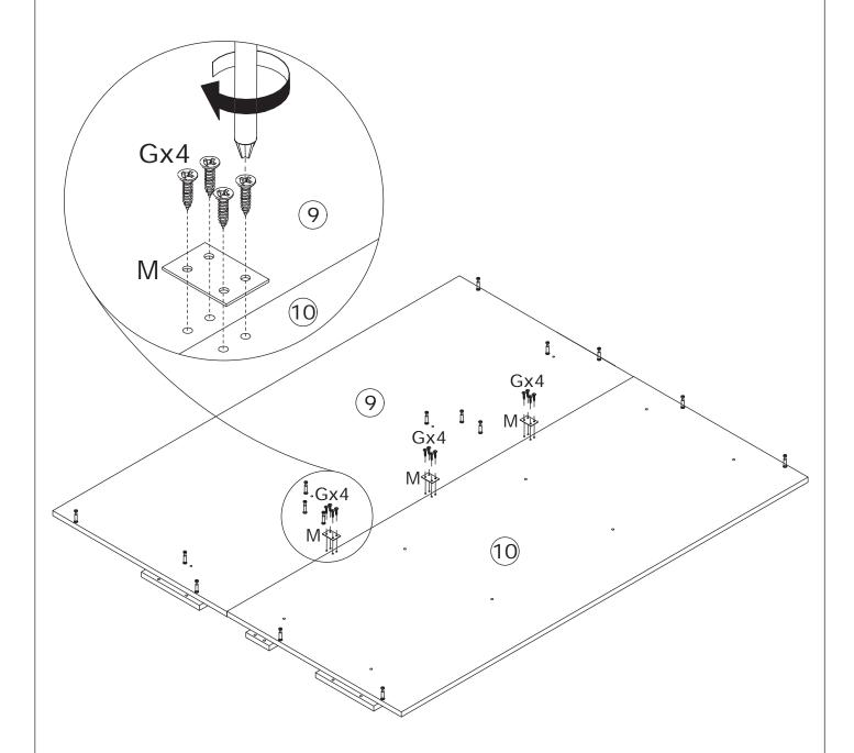
Fix iron sheet(M) to panel 9 and 10 with screw(G) as shown.
