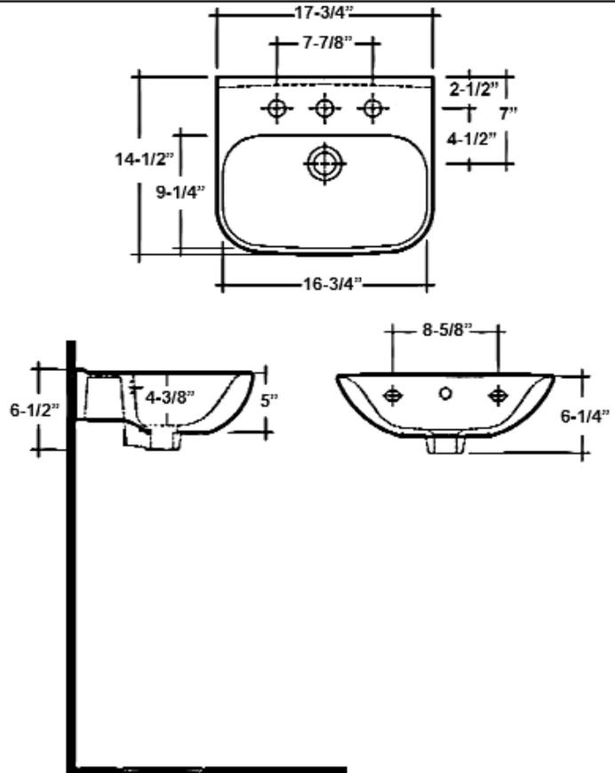
Dimensions of fixture are nominal and may vary within the range of tolerances established by ANSI Standard A112.19.2. Dimensions and specifications subject to change without notice.
