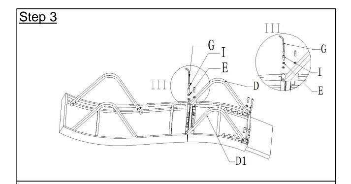
Attach Back Left Leg(D) to Seat(A) and Backrest(B) using Flat Washer(E) and Bolt(I) with Allen Key(G).
