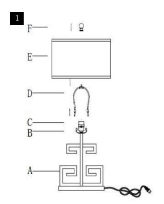
Step 1 Insert the Harp (D) into the Saddle (B). Put the shade(E) on the Harp(D),then tighten the Finial (F)into the Harp (D)
