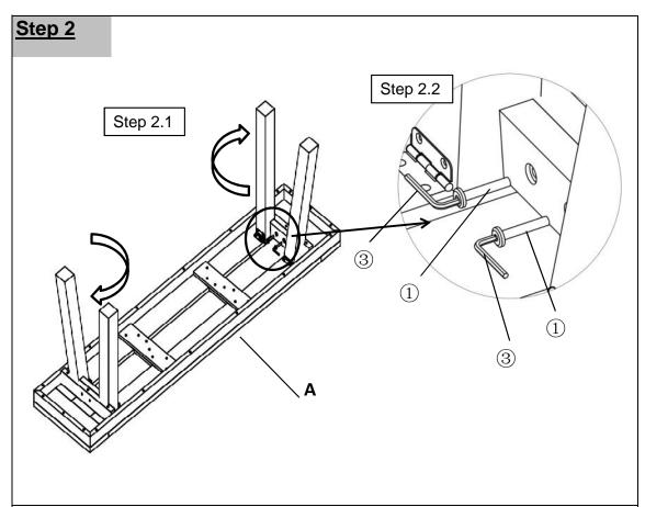
Place the Bench (A) facedown, onto a clean, soft surface to avoid any scratches or damage to the product.
