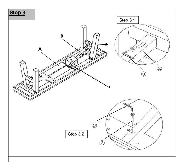
Position Leg Support Bar(B) as shown in picture above.
