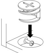
**EN\_**Quickfit head should be in the centre of the cam lock when the two panels are joined.
