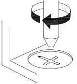
**EN\_**Turn cam lock clockwise to tighten.
