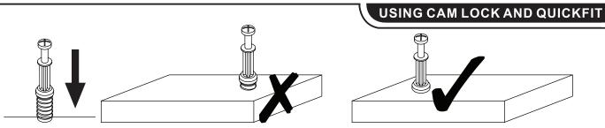
**EN\_QUICKFIT:**Tighten quickfit until shoulder is flush with panel.Do not overtighten or undertighten.
