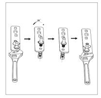
5. Moving the lower hinge across to the opposite side and fix into position. Place the door on to the pin of the lower hinge, note care must be taken as the door will be loose. Once this has been completed screw in the adjustable feet and the fit the small screw to the opposite side of the fridge.
