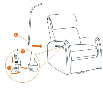
Connect the iPad Frame(E) or Mobile Frame(D) at the top of the Support Frame(C) until the connection is secure.
