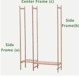
④ Secure Side frame (a) onto the Small Panel with Long Screws (q).
