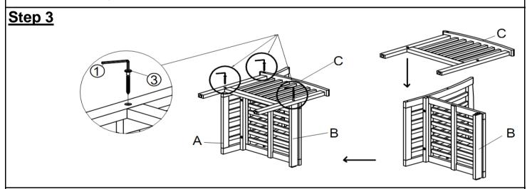
Attach Left Leg Panel (C) to Backrest Panel (A) and Seat Panel (B) using 3 Screws (3) + Allen Key (1).
