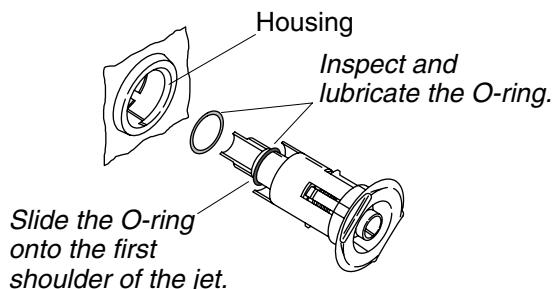
Insert the jet into the housing, and lightly push and rotate until it snaps in position.
