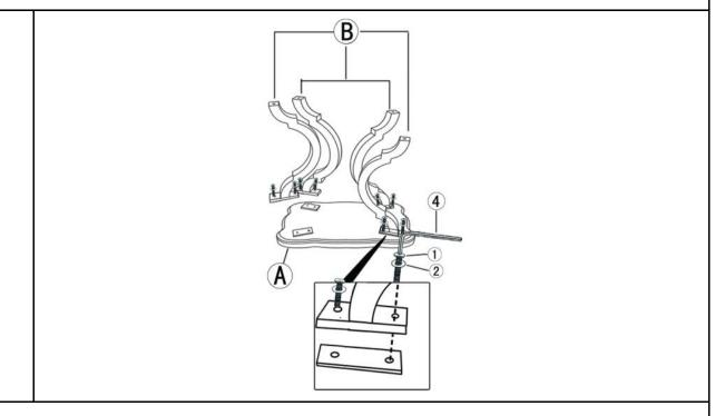
Place the Table Top(A) on a clean, non-marring surface, facedown. Attach Leg(B) to the Table Top(A) using Bolt(1) and Flat Washer(2) with Allen Key(4). repeat the same step to insert the remaining 3 legs.
