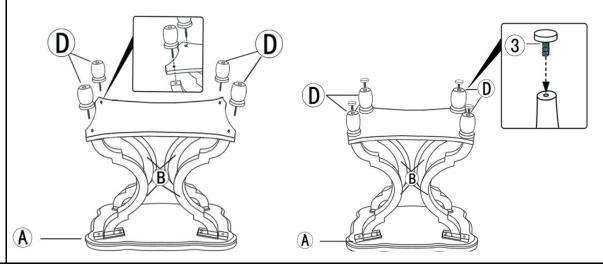
Slightly screw the Feet(D) one by one through the Shelf(C) to connect with the Leg(B).
