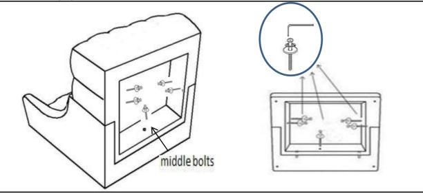
You should first fix the middle bolts on the Chair seat (B) tightly until there is no gap between Chair seat (B) and Chair backrest (A). Using hand to push Chair seat (B) forward a bit for finding and insert the bolts for sides correctly, and fix them.
