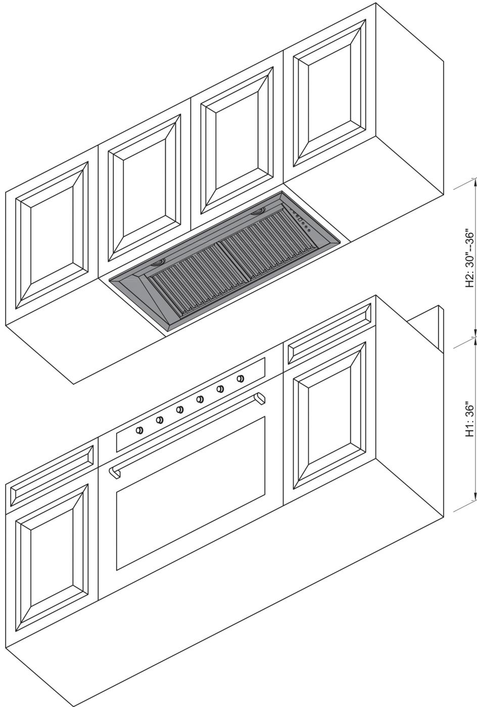
\*When installing a range hood insert, it is recommended to install the unit at a minimum of 30" from the cooktop.
