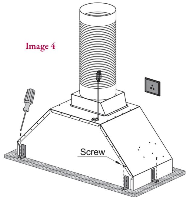
★ *Due to some installation differences with custom hoods the L brackets may not work. Before installing insert please determine if the insert will work for your installation needs. You may predrill holes into the insert unit to accommodate for custom hood installations.*
