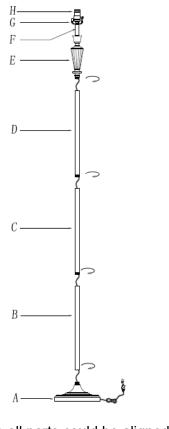
Make sure all parts could be aligned before assemble Do not rotate lamp body too hard avoid base screw broken Pull cord through lamp base(A) to tighten stem connections, Screw the tube (B) onto the base (A) Screw the tube (C) onto the tube (B) Screw the part (D) onto the tube(C) Screw the part (E,F,G,H) onto the tube(D) **ENJOY YOUR LAMP**
