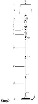
Insert the Harp (I) into the Saddle (G). Put the shade(K) on the Harp(I), then tighten the Finial (L) into the Harp (I) Insert the bulb(J) into the socket(H). Step3 Put the light on a level surface to check if everything is stable.
