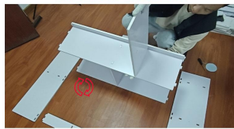
5. FLIP UP; ASSEMBLE G PLATE TO B PLATE
