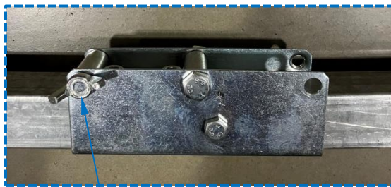
Wing-head bolt installed in first bolt hole
