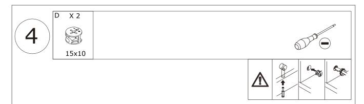
Attach plate 6 to plate 11, turn cam locks(D) clockwise to tighten as shown.
