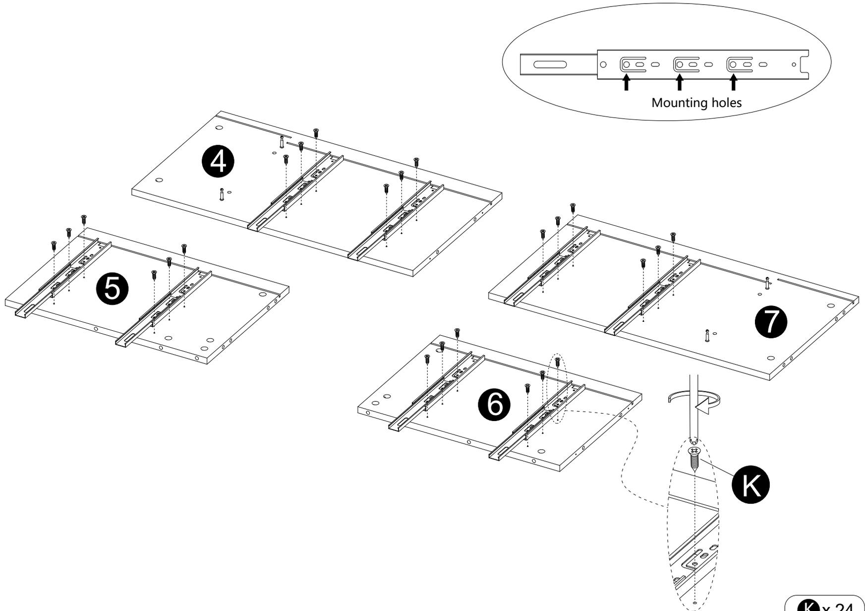
· Attach Slider arms to panels (4,5,6,7) with screws (K) correctly.
