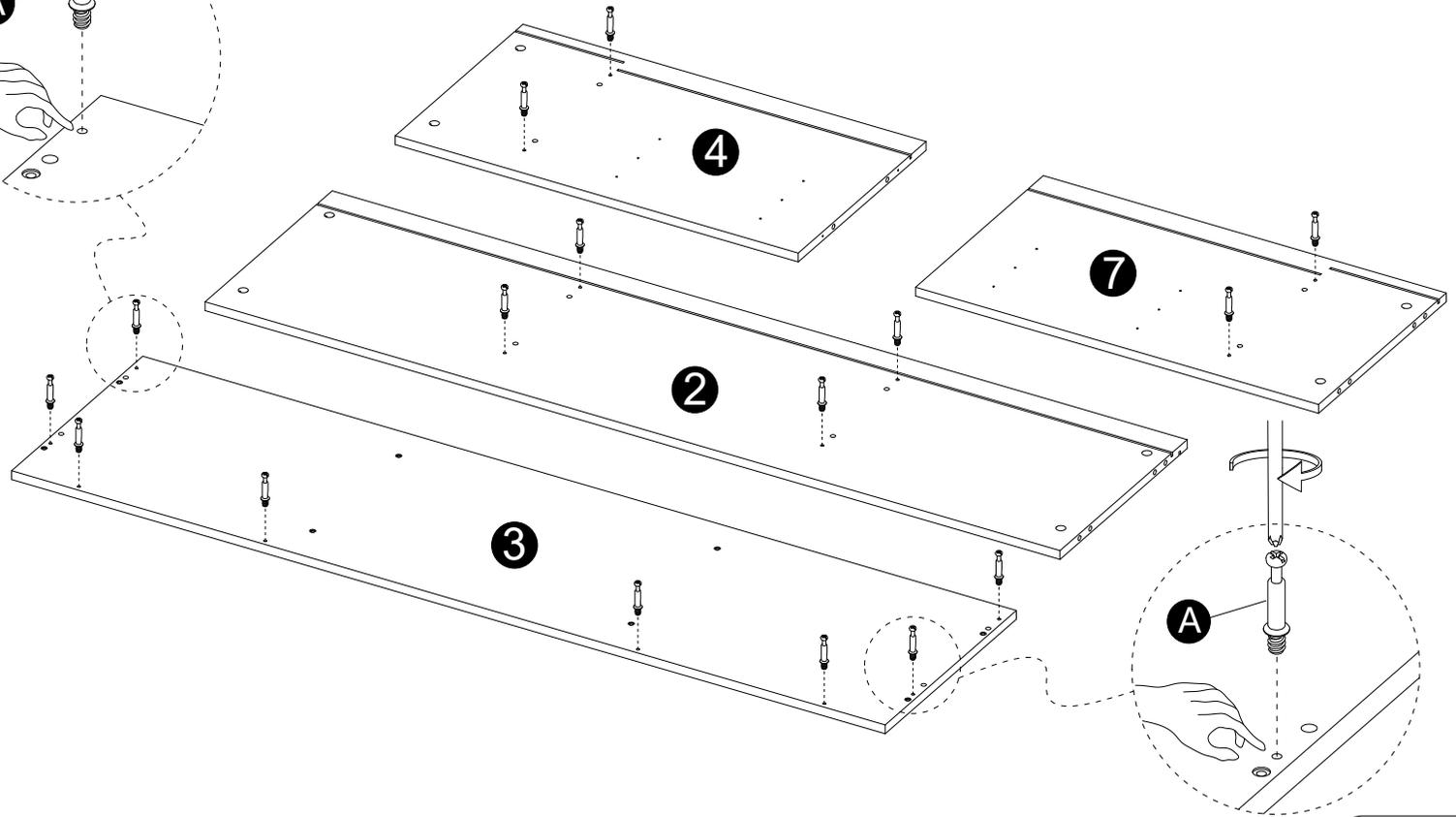
· Screw cam bolts (A) into panels (2,3,4,7).
