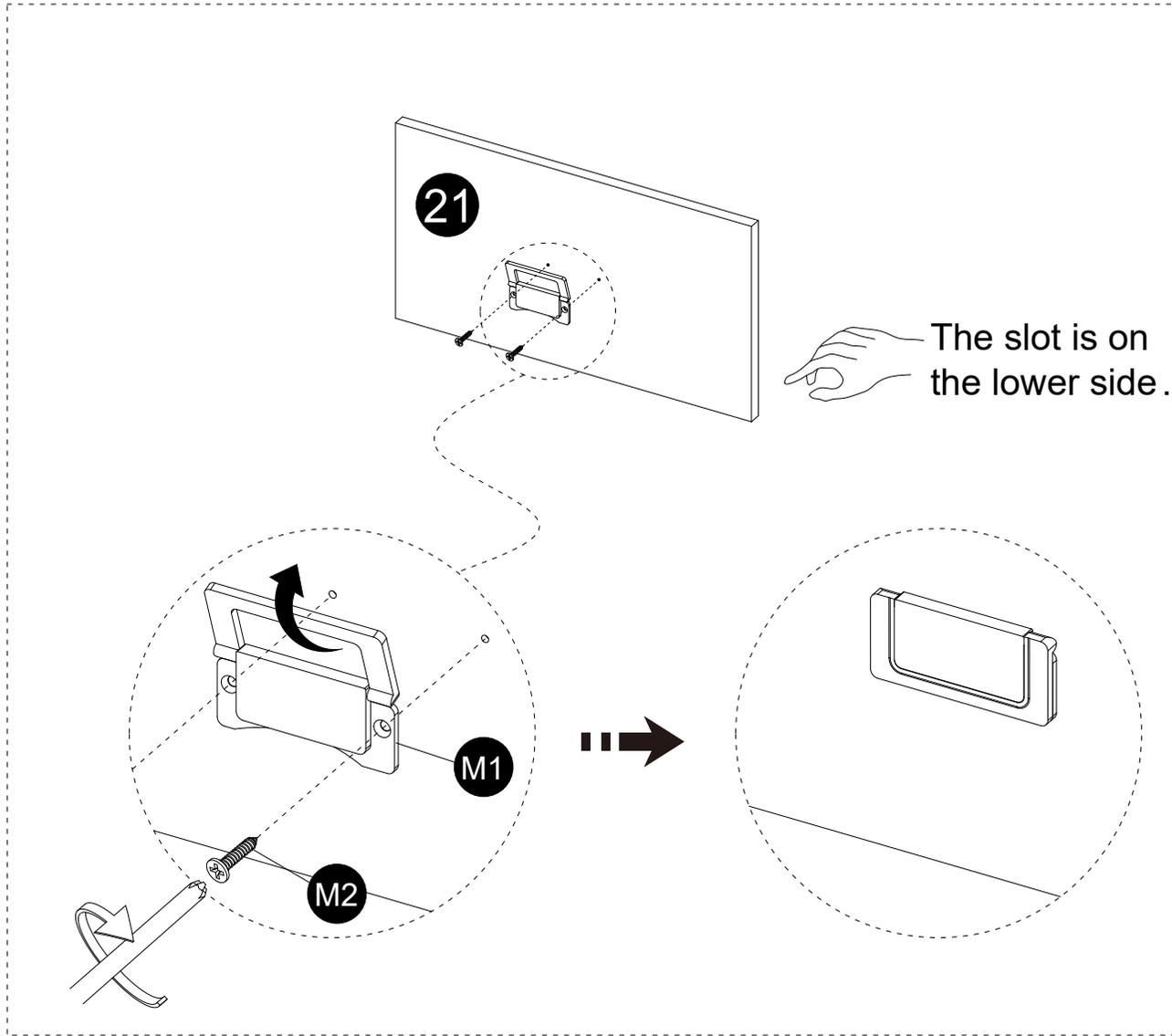
· Attach parts (M1) to panels (21) with screws (M2).
