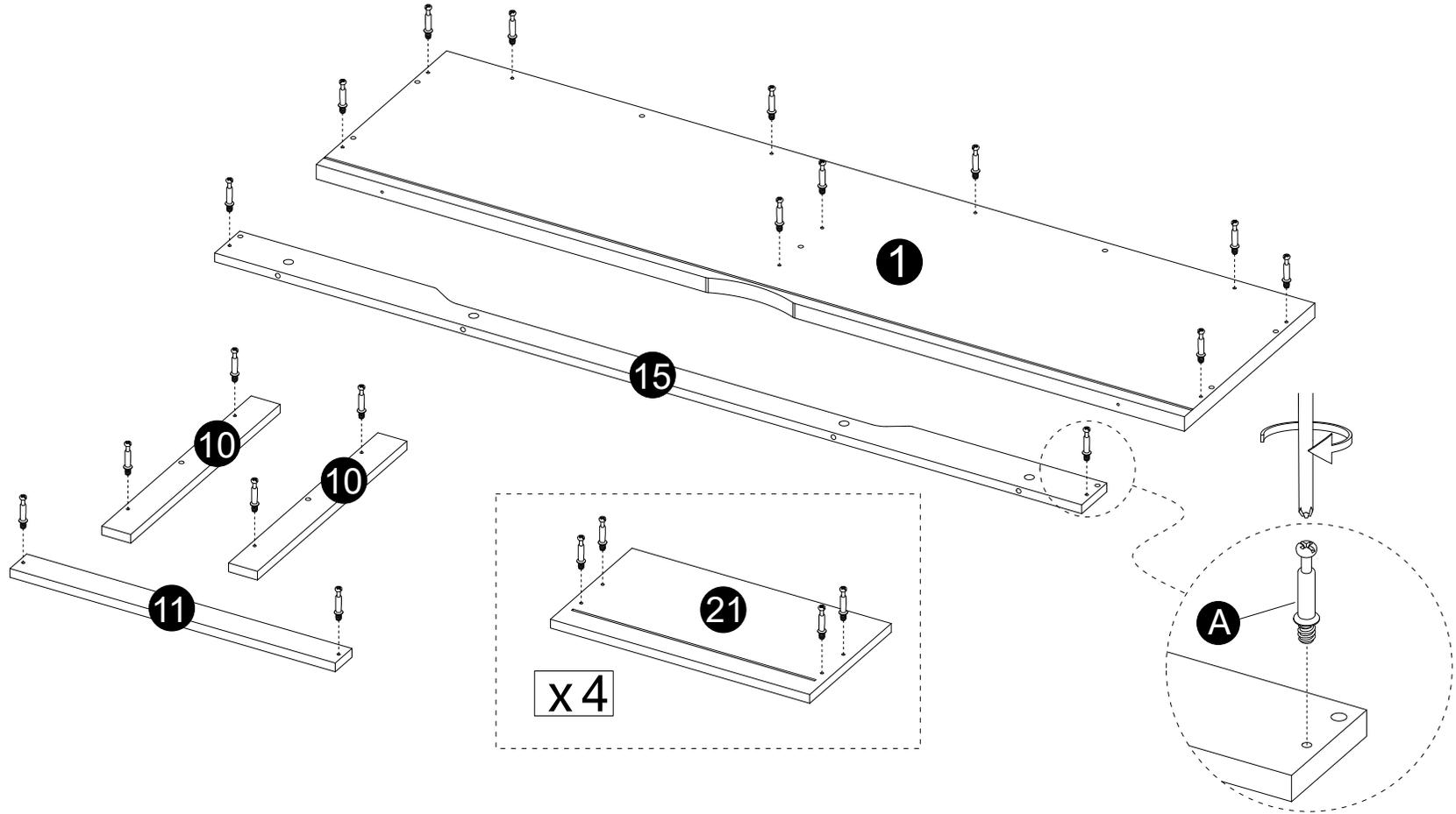
· Screw cam bolts (A) into panels (1,10,11,15,21).
