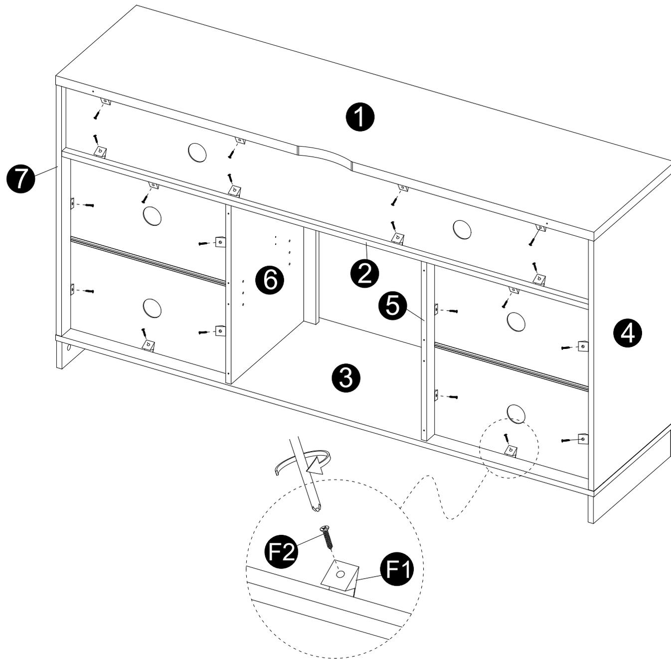
· Secure parts (F1) with screws (F2) as per diagram.
