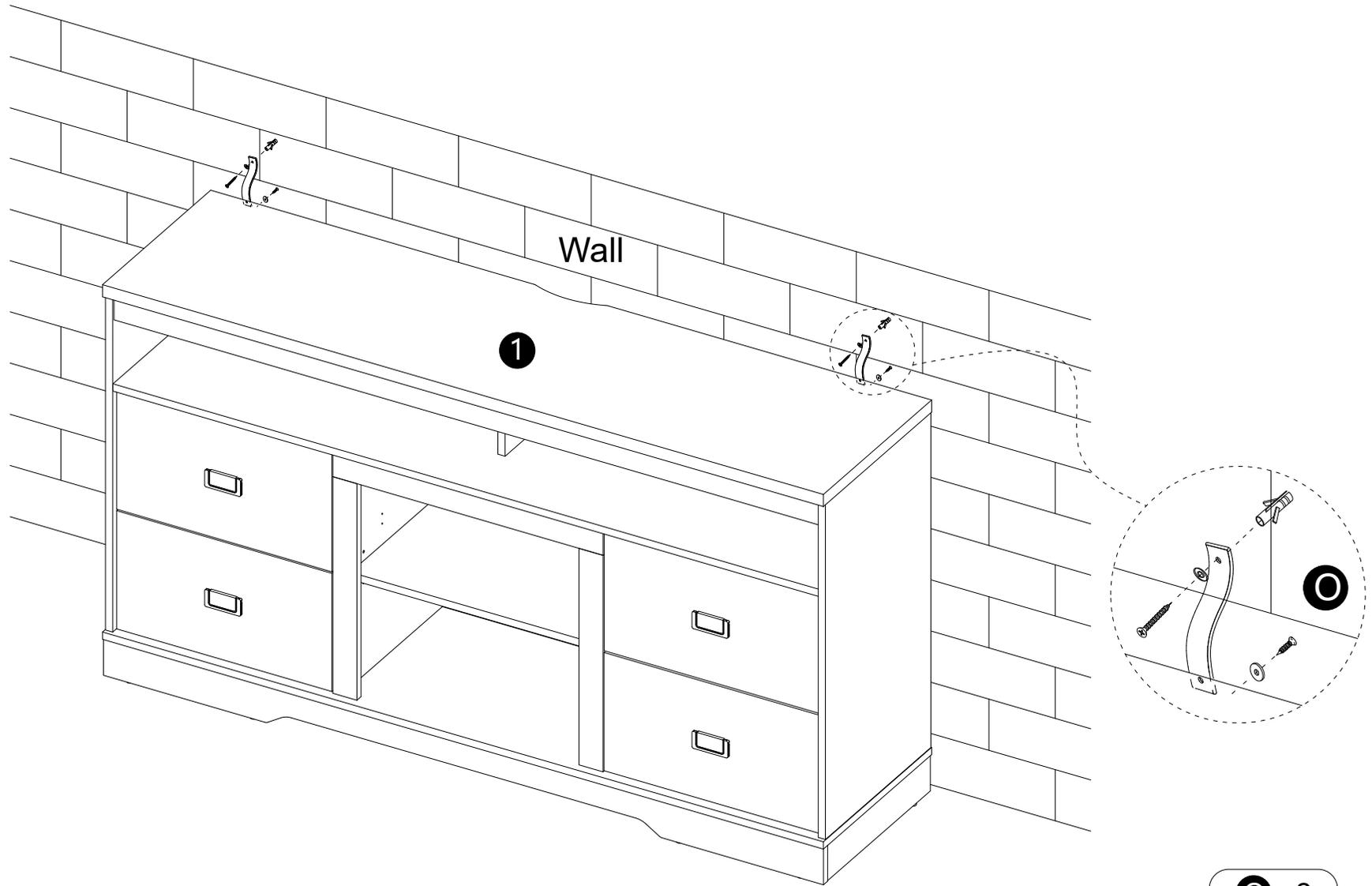
· To prevent TV cabinet from toppling,install the parts (O).
