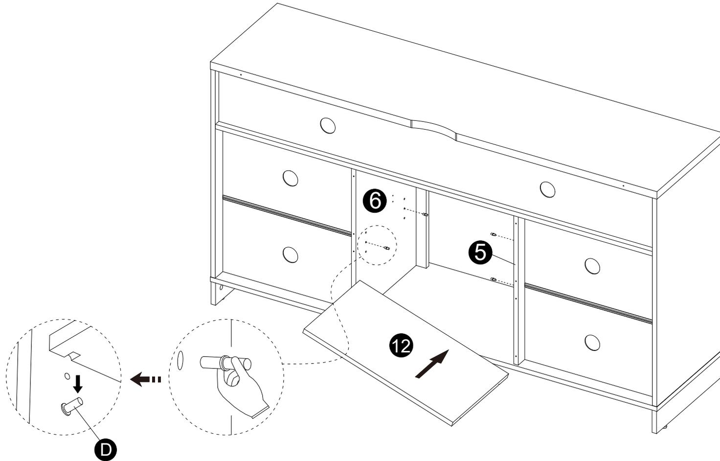
· Attach panel (12) to panels (5,6) using parts (D).
