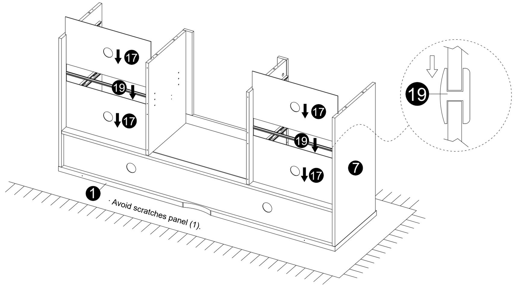
· Carefully slide parts (17,19) into place along the back of the assembly.
