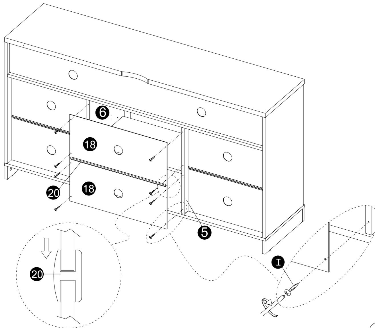
· Attach parts (18,20) to panels (5,6) with screws (I) correctly,
