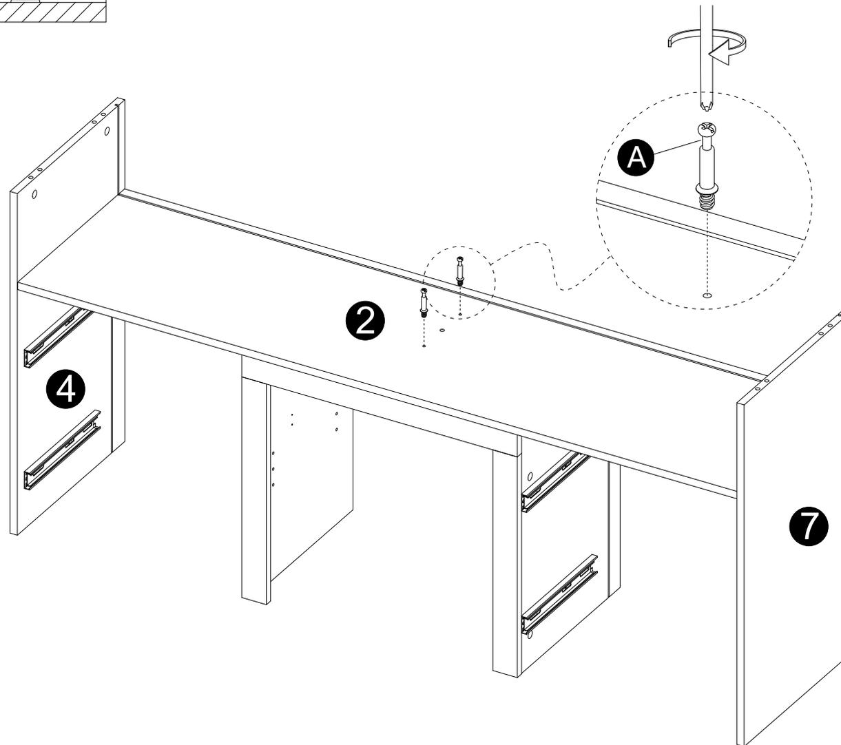
· Screw cam bolts (A) into panel (2).
