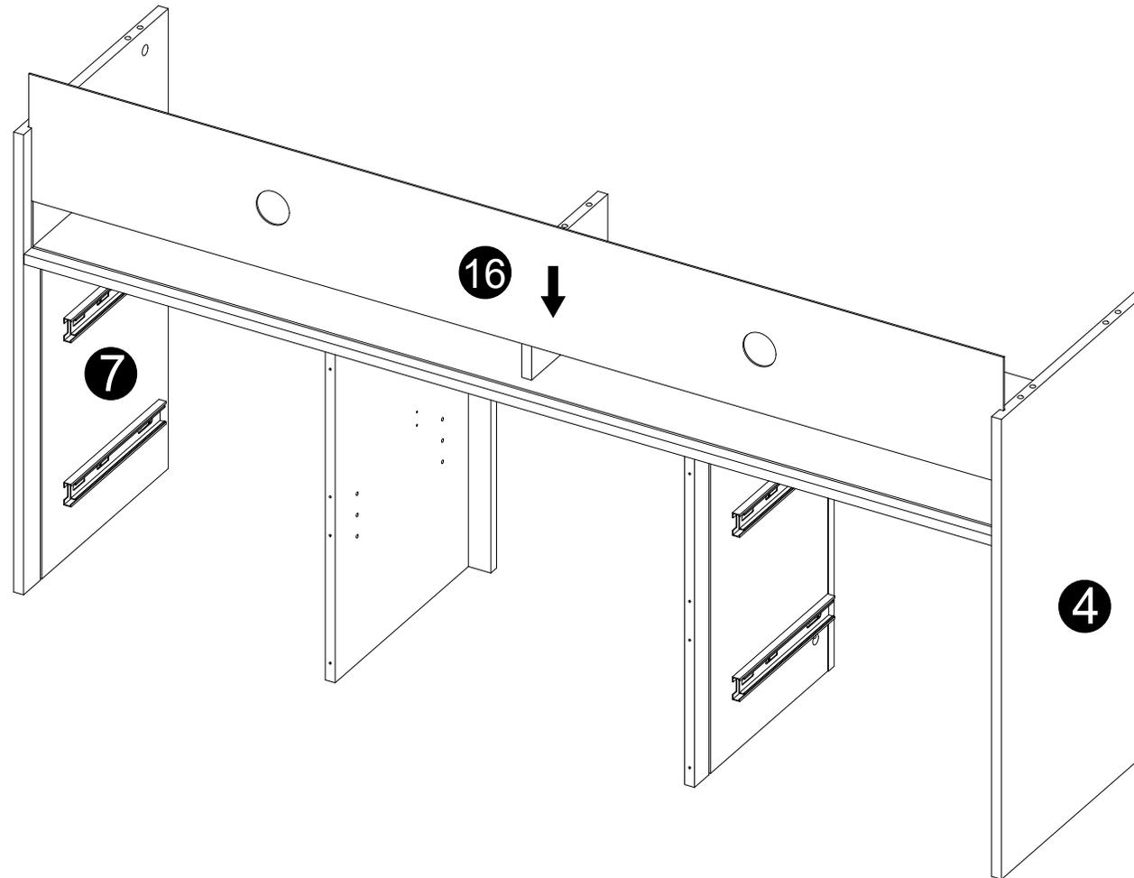
· Carefully slide part (16) into place along the back of the assembly.
