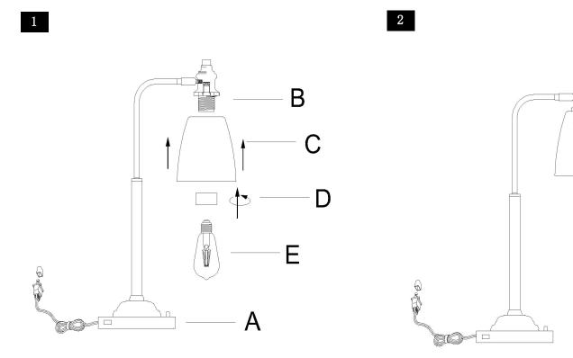
Step 1 Put the shade (C) on the Socket (B),then screw the Metal ring (D) onto the Socket (B) Insert the bulb (E) into the socket (B). Step2 Put the light on a level surface to check if everything is stable.
