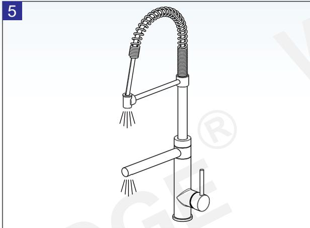
5 After installation is complete, remove Spray head and rotate handle to the close position. Turn Water Supply Valves on, and check all connections for leak. Flush faucet by running hot and cold water in full position for one minute.
