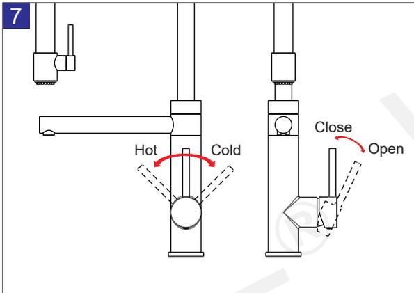
7 Lift the handle up, the cartridge will be activated allowing water to flow. The water flow will increase by continuing to rotate handle. By rotating the handle to the right, the water temperature will decrease to cold flow only. By rotating Handle to the left, the water temperature will increase to hot only.
