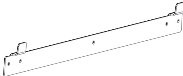
Fix the supporting bracket with at least 5 screws horizontally to the wall, use the appropriate fixings for the type of wall - Note the unit is heavy approximately 55lbs.
