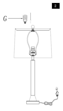
Step2 Insert the bulb(G) into the socket(C).
