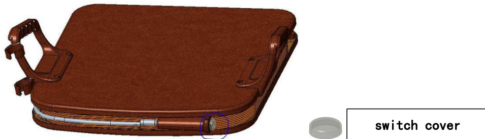
Figure.8 Remove the switch cover
