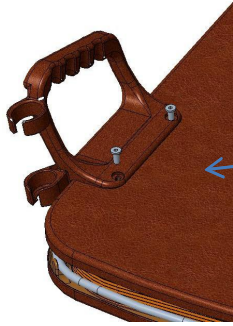
Figure.6 Installation of armrest cover
