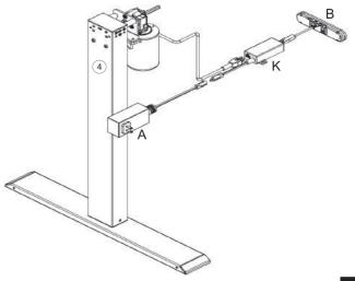
Use D -Wire Clips to tidy up the wires.
