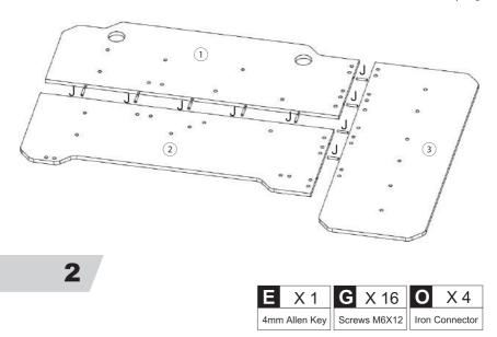
Note: The horizontal bar on the Iron Connector should be perpendicular to the seam of the table panel splice
