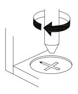
Turn cam lock clockwise to tighten.
