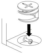
Quickfit head should be in the centre of the cam lock when the two panels are joined. Cam lock should be inserted before quickfit.
