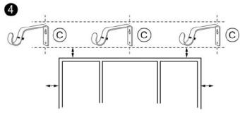
Repeat steps 2-3 for additional bracket(s). It is recommended to use a center bracket for expansions over 48". Use level if necessary.
