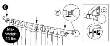
Place drapery panels (not included) onto drapery rod and extend to desired length. Hang rod on brackets. Insert finial (E) into the end of the rod and tighten the set screws on the brackets (C).
