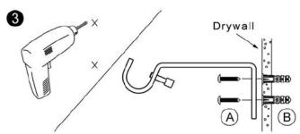
Drill pilot holes into wall with 1/4" drill bit (not included).
