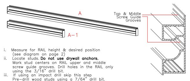
iv. Anchor the RAIL to the wall using the #10 x 2" wood screws (H) provided. Do not over tighten as RAIL can bend. Secure the top center screw first. IMPORTANT — Make sure the RAIL is level before drilling mounting holes. If the RAIL is not level the system will not function properly. Then attach the remaining screws.
