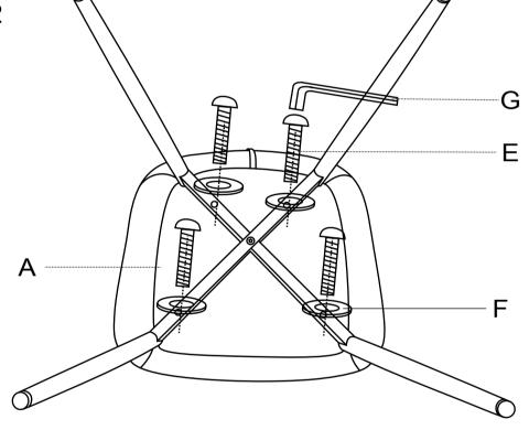
Insert the screws in the holes and tighten item to 100%.
