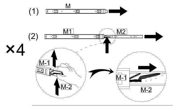
Move the black paddle upward and pull out (M2) to the right.
