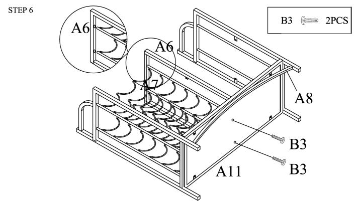
Insert Bottle Rack(A7) into holes on the top of Divider Frame (A6). Then Attach Bottle Rack (A7) and Divider Frame (A6) to Bottom Panel (A11) using Bolts (B3). NOTE: Please do not tighten Bolts (B3) until step 9.
