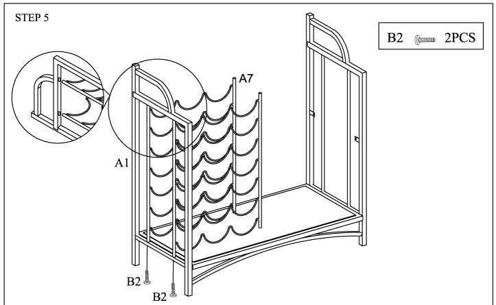
Insert Bottle Rack (A7) into holes on top of Left Side Frame (A1), Then assemble Bottle Rack (A7) to the bottom of Left Side Frame (A1) using Bolts (B2).
