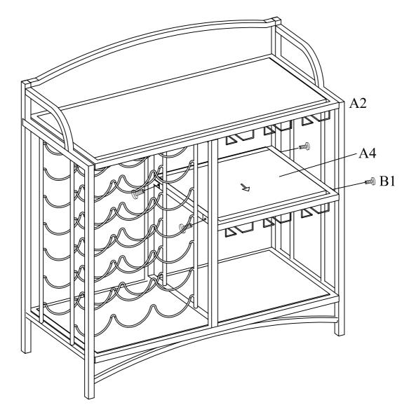
Assemble Shelf Frame A4 to Right Side Frame A2 and Divider A6 using Bolts (B1). Then tighten all bolts at this point.
